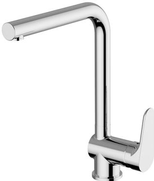
**FEATURES:** MADE IN ITALY, single-control sink mixer, brass chrome plated body, modern design, pull-out shower, lateral lever, cartridge Ø 40 mm short, aerator M22x1, stainless steel flexible pipe M10x1, length 370 mm, G3/8" F connection, fixing set M32x1.5, extension for fixing set, 5 years warranty, carton box single packed.
