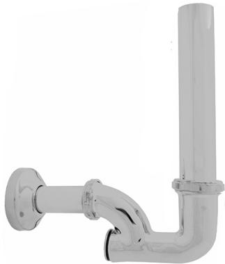
**FEATURES:** MADE IN ITALY, brass chrome plated column trap for wash basin with inspection cap, 1 1/4" connection, inlet pipe Ø 32 mm length 75 mm, outlet pipe Ø 32 mm length 250 mm, stainless steel rosette Ø 75 mm, 5 years warranty, carton box single packed.
