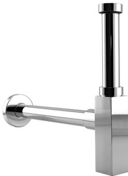
**FEATURES:** MADE IN ITALY, basin brass chrome plated bottle trap, 1 1/4" connection, inlet pipe Ø 32 mm length 230 mm, outlet pipe Ø 32 mm length 300 mm, brass chrome plated rosette Ø 80 mm, bottom inspection plug, 5 years warranty, carton box single packed.
