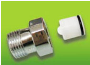
**FEATURES:** MADE IN ITALY, ABS chrome plated fitting,  $\frac{1}{2}$ " M x  $\frac{1}{2}$ " F connection, water saving 8 lt/min, white color, POM, rubber gasket  $\frac{1}{2}$ ", 5 years warranty, plastic bag single packed.
