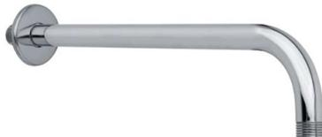
**FEATURES:** MADE IN ITALY, modern design, wall mounted shower arm, brass chrome plated round shape Ø 21 mm, 1/2" M x 1/2" M connection, stainless steel Ø 50 mm round rosette, 5 years warranty, plastic bag single packed.
