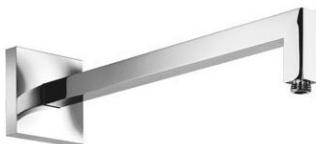
**FEATURES:** MADE IN ITALY, modern design, wall mounted reinforced shower arm brass chrome plated, square shape 25 x 25 mm, 1/2" M x 1/2" M connection, ABS chrome plated 100 x 100 mm square rosette, 5 years warranty, carton box single packed.
