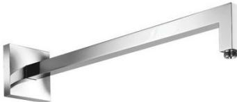
**FEATURES:** MADE IN ITALY, modern design, wall mounted reinforced shower arm brass chrome plated, square shape 25 x 25 mm, 1/2" M x 1/2" M connection, ABS chrome plated 100 x 100 mm square rosette, 5 years warranty, carton box single packed.
